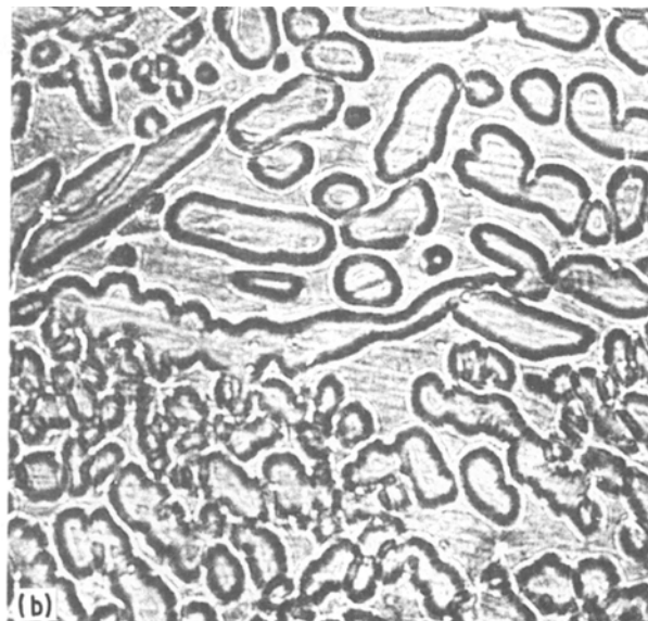
Figure 1 Microstructures of homogenized (at 1100° C) samples of (a) alloy 1A (5Al, 0.3C); (b) alloy 3A (10Al, 0.3C); (c) alloy 3C (10Al, 0.9C). Magnification 200 × .
